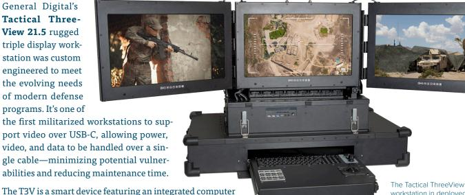
system that connects to a server through a gigabit Ethernet
