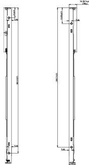
Figure 4: Display dimensions (unit of measure: mm; tolerance is ±0.50 mm unless otherwise indicated)
