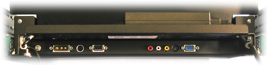
Rear View of SL2-19W Showing Power Supply and Interface Connectors
