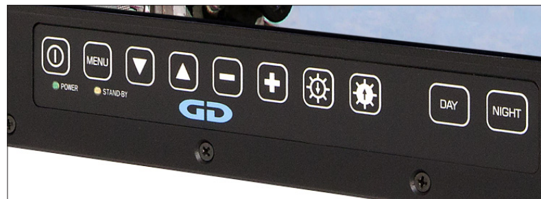
Silicone keypad close-up showing individual buttons for Daylight Mode and NVIS Mode
