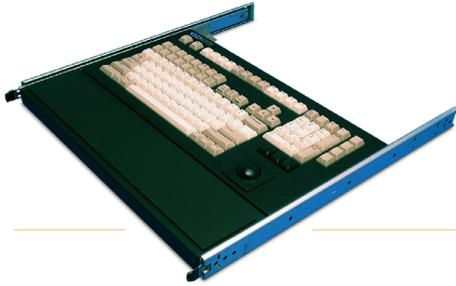
This rugged spill-/dust-proof keyboard features solid-state, full-travel keys. Configurable for PS/2 or USB compatibility. Housed in an aluminum NEMA12 enclosure. Standard equipment includes 1-3/8" trackball pointing device with 3 mouse buttons.
