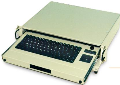
With 101-key functionality and enclosed in a sealed aluminum NEMA 4X 2U enclosure, this ruggedized keyboard features silicone rubber keys, backlight dimmer with auto-shutoff, sealed trackball with 3 mouse buttons. PS/2 or USB configurable.
