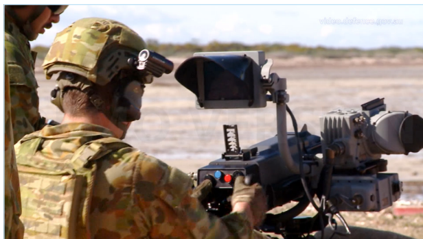
Mounted 6.5" Barracuda with optional rubber hood
