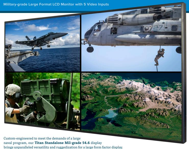
End-user certified to MIL-DTL-901, MIL-STD-167 and -461 for shock, vibration, and EMI, this Titan model is the ideal choice for mission briefing rooms and other tactically collaborative environments. It features a number of options for data and video inputs/outputs, as well as integrated speakers.
