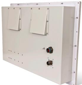
Mil-spec Saber PanelMount 24.0 includes a ½" thick front bezel, mil-grade connectors, and rear louvers to protect fans
