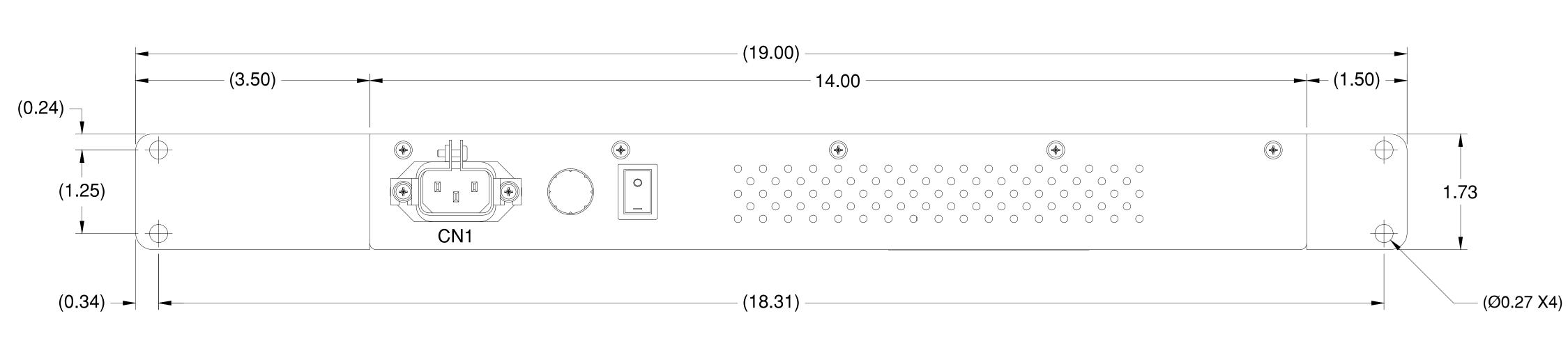
NOTE: DIMENSIONS IN PARENTHESIS REPRESENT THE 19" RACK MOUNT KIT WHEN INSTALLED ON THE POWER SUPPLY.
