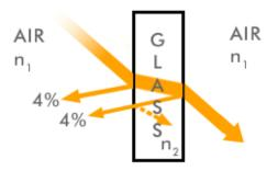
The Fresnel reflection for non-polarized light is related to the refractive index by the following equation<sup>1</sup>:
