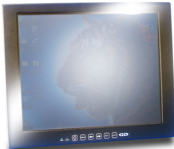
Standard LCD Monitor in High Ambient Light Environment without Optical Enhancement
