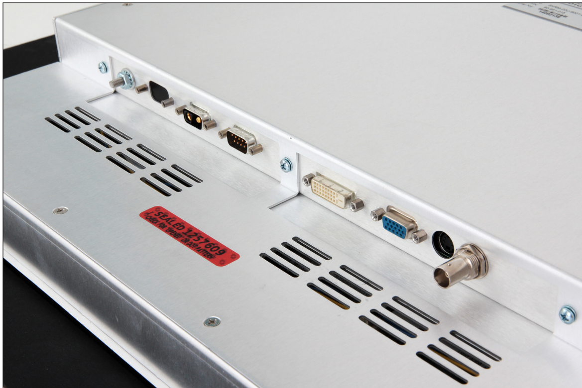
Rear View of Saber RackMount Solar/NVIS 19.0 Showing Interface Connectors
