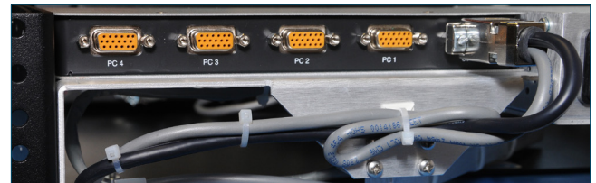
The 4-port KVM Switch integrates perfectly on the rear mounting bracket beside the optional 1U power supply
