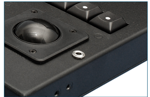
The SlimLine 1U Audio includes a 3.5 mm headphone jack next to the trackball
