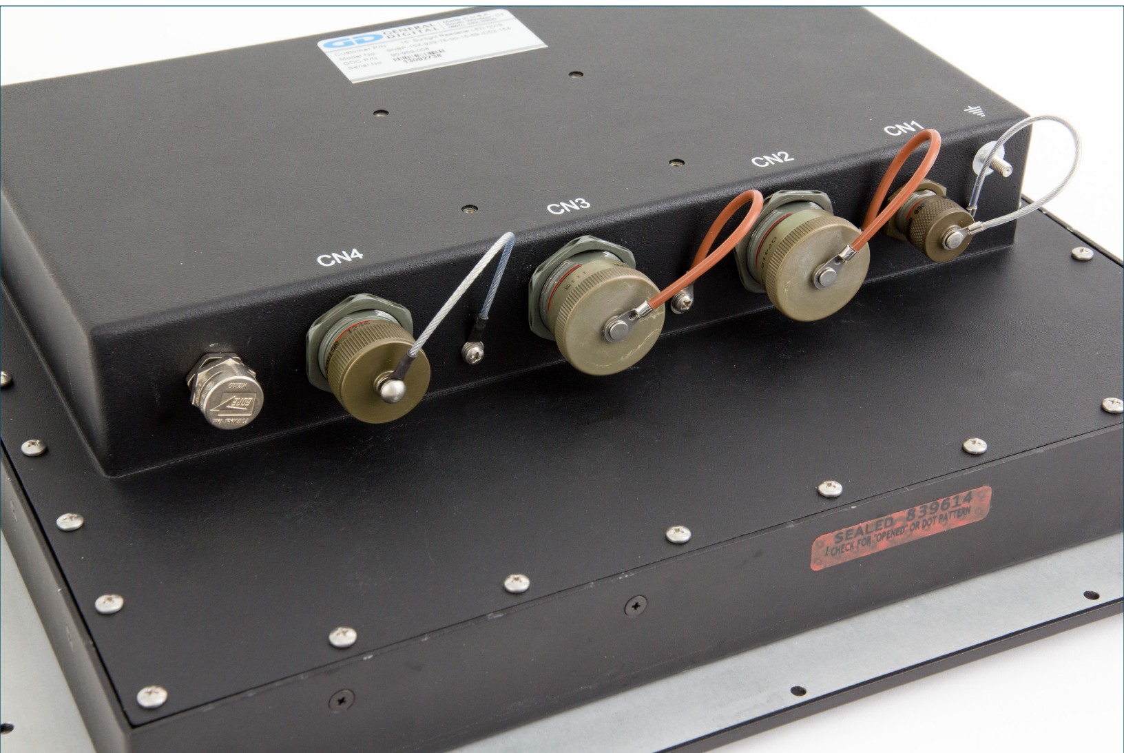
Rear view showing GORE® vent and sealed circular military connectors
